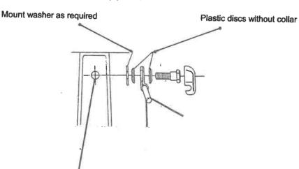
Remove threaded plug or punch holes in the paneling at the installation thread and mount parts as shown in the illustration
